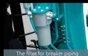
The filter for breaker piping
