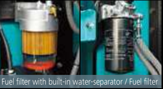
Fuel filter with built-in water-separator / Fuel filter
