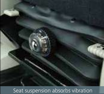
Seat suspension absorbs vibration
